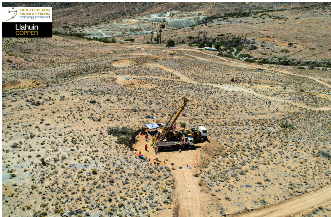
Figure 1. RC rig in action at Cerro De Oro, with Central Porphyry workings in the centre background
