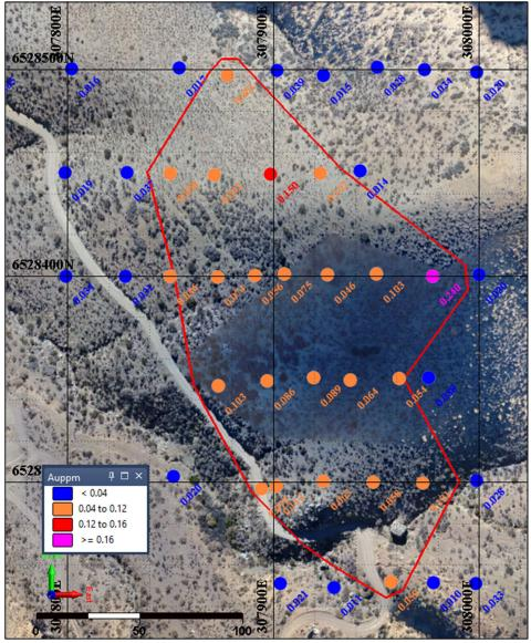
Figure 4 New +40ppp Gold in Soil Anomaly (peak value 240ppb Gold) in the Southern part of the Llahuin Project
