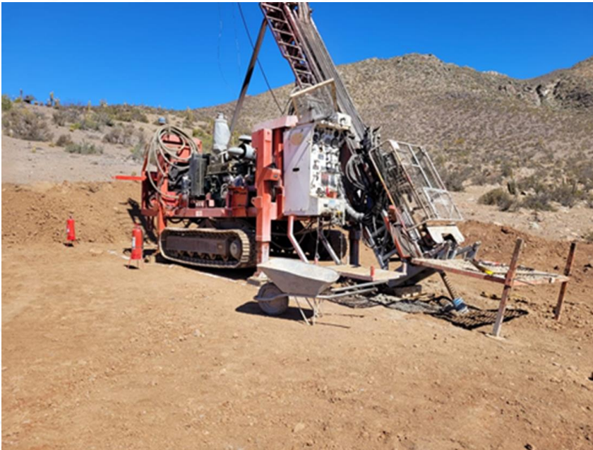
Diamond drill rig in operation at Colina2
